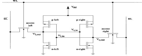
Figure 1. 6T-SRAM-AAM circuit diagram.
