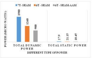
Figure 4. Comparison performance of total dynamic and static power for SRAM design in 22 nnm technology
