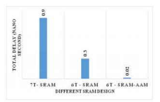
Figure 5. Comparison of total delay performance for 22 nm technology
